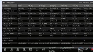
Scrolling horizontally allows the user to see and compare the various embedded audio groups for each of the audio signals present. AES Channel status provides syntax information for parameters such as Emphasis, Locking of Source, Sampling Frequency, Channel Mode and Audio Word Length.
